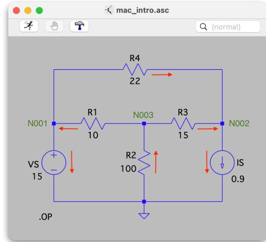
The second method for viewing the DC results works well if we are primarily interested in the node voltages. LTspice will print the node voltage right on the circuit schematic, similar to what we might do if analyzing the circuit with pencil and paper.
