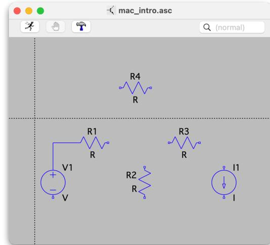
Continue wiring to connect all the other components according to the original circuit diagram. A wire can be started or stopped on an existing wire to make a T-connection, which is indicated by a small square dot. (Similar to the circular dots used to show connections on circuits in class.) To get out of wiring mode, hit the “escape” key.
