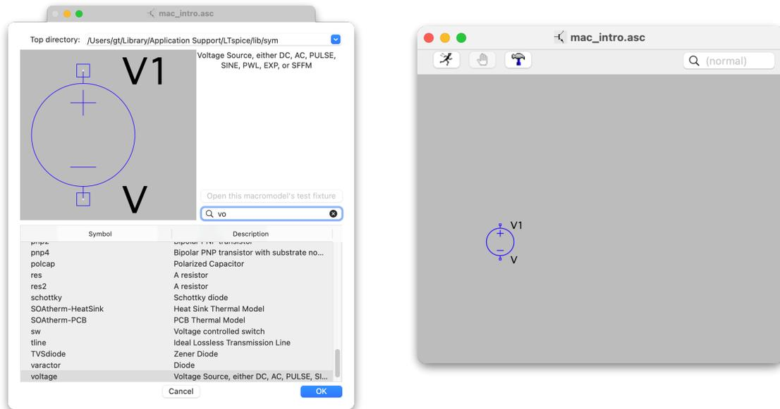
After placing the first voltage source, the cursor still has a source icon attached to it. We could place more sources if we wanted, but since we need only one, hit the escape key. This takes us out of “voltage-source placement mode” and the source icon disappears.
