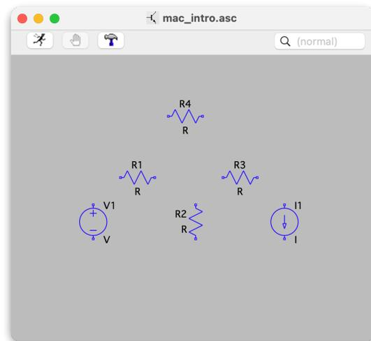
5. Wire the components together using the wire tool. Right-click and choose “Draft→Wires” from the pop-up menu. The cursor turns into a giant pair of cross-hairs that extend horizontally and vertically across the entire window. These are helpful in aligning the placement of the wires.
