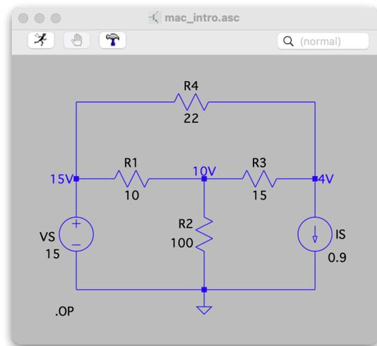
Unfortunately, the macOS version seems to be lacking a similar method for displaying currents.<sup>3</sup> If needed, we can use the node voltages and KCL to calculate a branch current.
