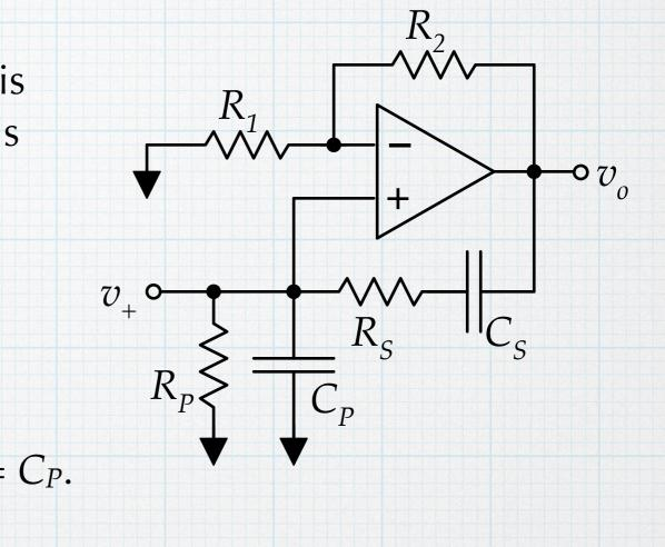
$$v_{+} = \frac{Z_{p}}{Z_{p} + Z_{s}} v_{+} = \frac{\frac{R_{p}}{1 + sR_{p}C_{p}}}{\frac{R_{p}}{1 + sR_{p}C_{p}} + R_{s} + \frac{1}{sC_{s}}} = \frac{1}{1 + \frac{R_{s}}{R_{p}} + \frac{C_{p}}{C_{s}} + sR_{s}C_{p} + \frac{1}{sR_{p}C_{s}}} v_{o}$$
