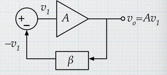
Furthermore, if the circuit has this instability in the loop frequency response, it is guaranteed to oscillate. Any disturbance in a circuit (a bit of noise, a switch closing, etc) will induce a voltage somewhere along the path of the circuit. That disturbance will probably have a component at  $\omega = \omega_{180}$ . That component will be sustained by the positive feedback at that frequency.
