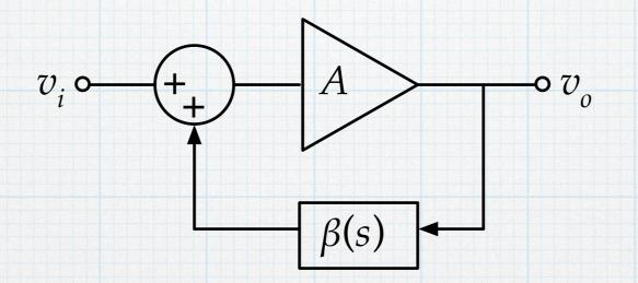
The feedback network has a very specific frequency dependence,  $\beta \rightarrow \beta(s)$ . With positive feedback, the closed-loop transfer function is
