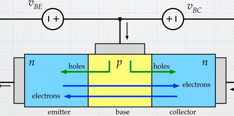
In saturation, there are many more carriers flowing across the two junctions. The base current is increasing because of the additional injection of holes into the collector. The net collector current is decreasing because of the opposing electron flow from collector to emitter.
