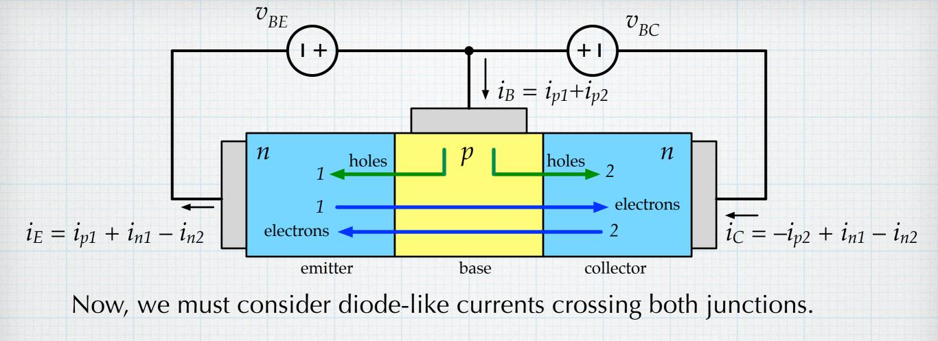
electrons injected emitter to base:
