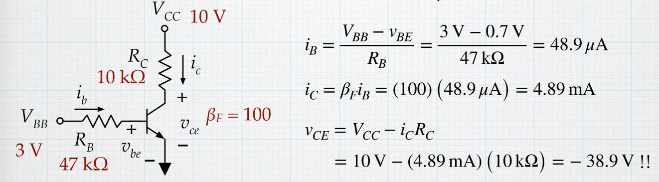
Red alert! Red Alert! Something is seriously wrong here —  $v_{CE}$  is extremely negative, which is not at all compatible with the B-C junction being reverse-biased. Furthermore, there is no way that we could get 39 V across any two points in the circuit when there is only one 10-V source and one 3-V source.
