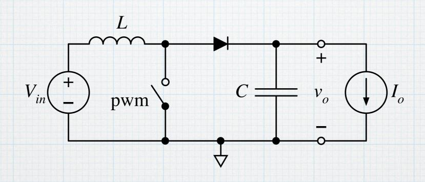
To get an initial view of the how a boost converter functions, we use the same assumptions — ideal components, PWM control of the switch, and constant values for  $V_{in}$  and  $v_o$  (with  $v_o > V_{in}$ ) — and the same steady-state approach as the buck converter. Look at the switch-closed and switch-opened situations.
