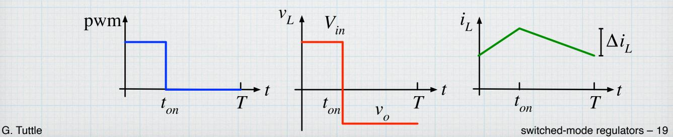
It's the same story. The power flow must balance — energy is added to the inductor when the switch is closed, and that energy is transferred to the capacitor and load when the switch is open.
