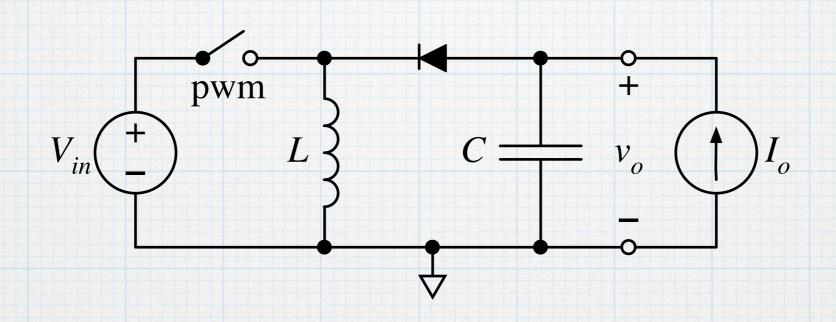
Note the change in the direction of the load current to be consistent with a negative output voltage.
