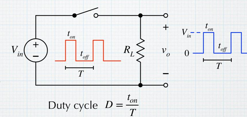
Add a low-pass filter it to remove the high-frequency parts, leaving only the DC.  $V_{in} + t_{on} + t_{off} + C + R_L > v_o + v_o + v_o = \frac{t_{on}}{T} \cdot V_{in} = D \cdot V_{in}$
