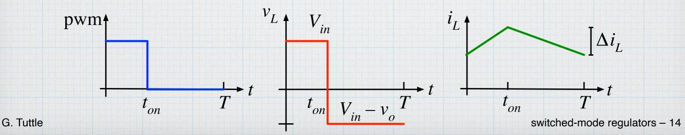
As with the buck converter, if the boost converter is in steady-state operation, the power flow must balance. Energy is added to the inductor when the switch is closed, and that energy is transferred to the capacitor and load when the switch is open.
