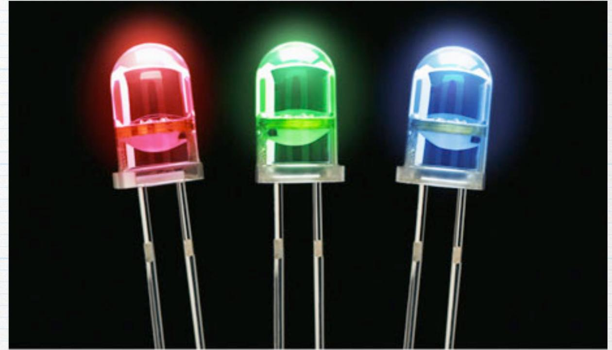
Using an LED is very simple, but there are a couple of precautions. First, you must *always* have a resistor in series with it. Without the resistor, you run the risk of having the diode current become too high, causing the diode to burn out. The value of the resistor is not critical — anything between  $100\ \Omega$  and  $1\ \text{k}\Omega$  is probably OK, although lower resistance values will give a brighter output.
