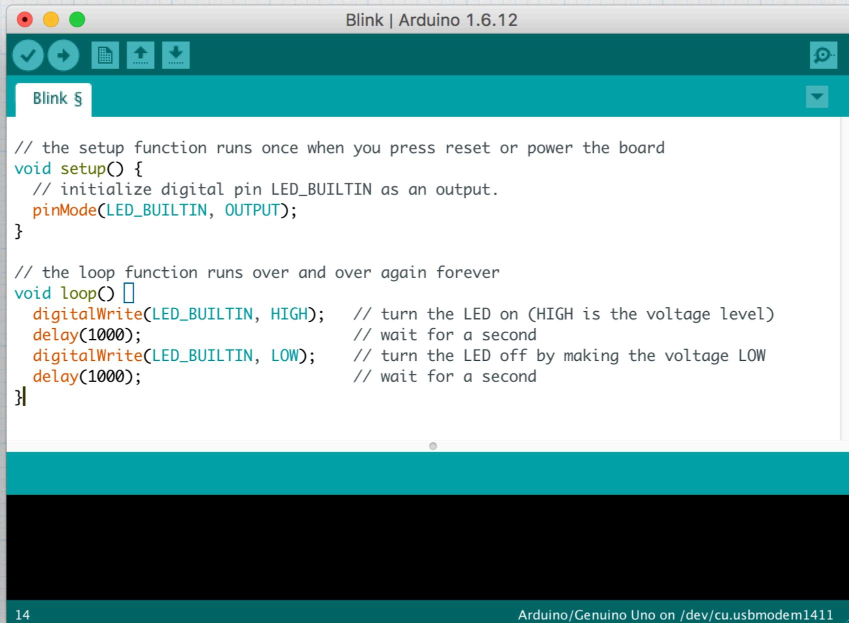
A screenshot of the Arduino IDE interface. The title bar reads "Blink | Arduino 1.6.12". The main window contains the following C++ code:
