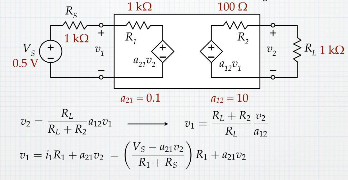
$$\frac{R_L + R_2}{R_L} \frac{v_2}{a_{12}} = \left(\frac{V_S - a_{21}v_2}{R_1 + R_S}\right) R_1 + a_{21}v_2 \qquad \text{Solve for } v_2.$$
