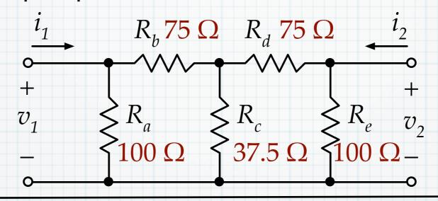
1. Apply a test voltage at  $v_1$ . Short circuit  $v_2$ . ( $R_e$  is shorted out.) Calculate the terminal currents.
