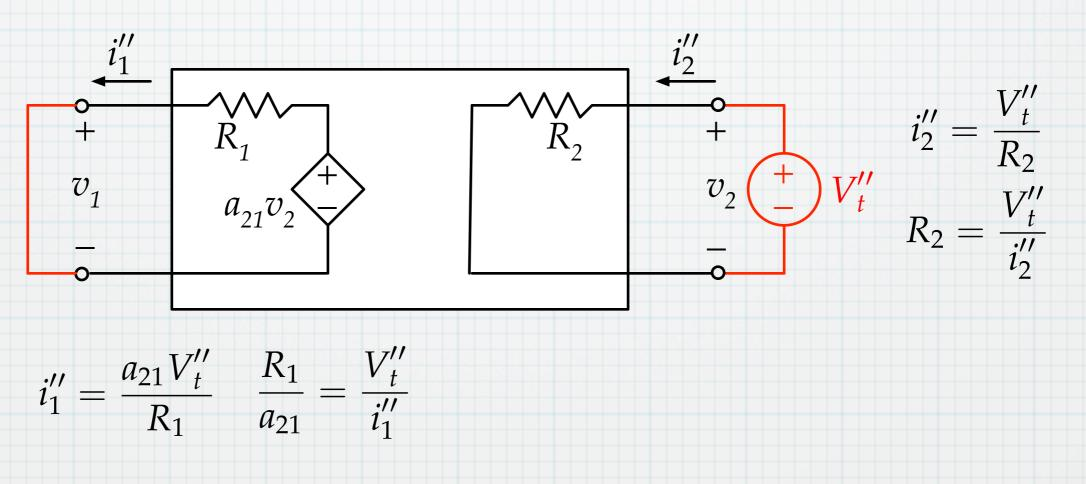
From the measured (calculated) values, we can determine the four parameters for the two-port.
