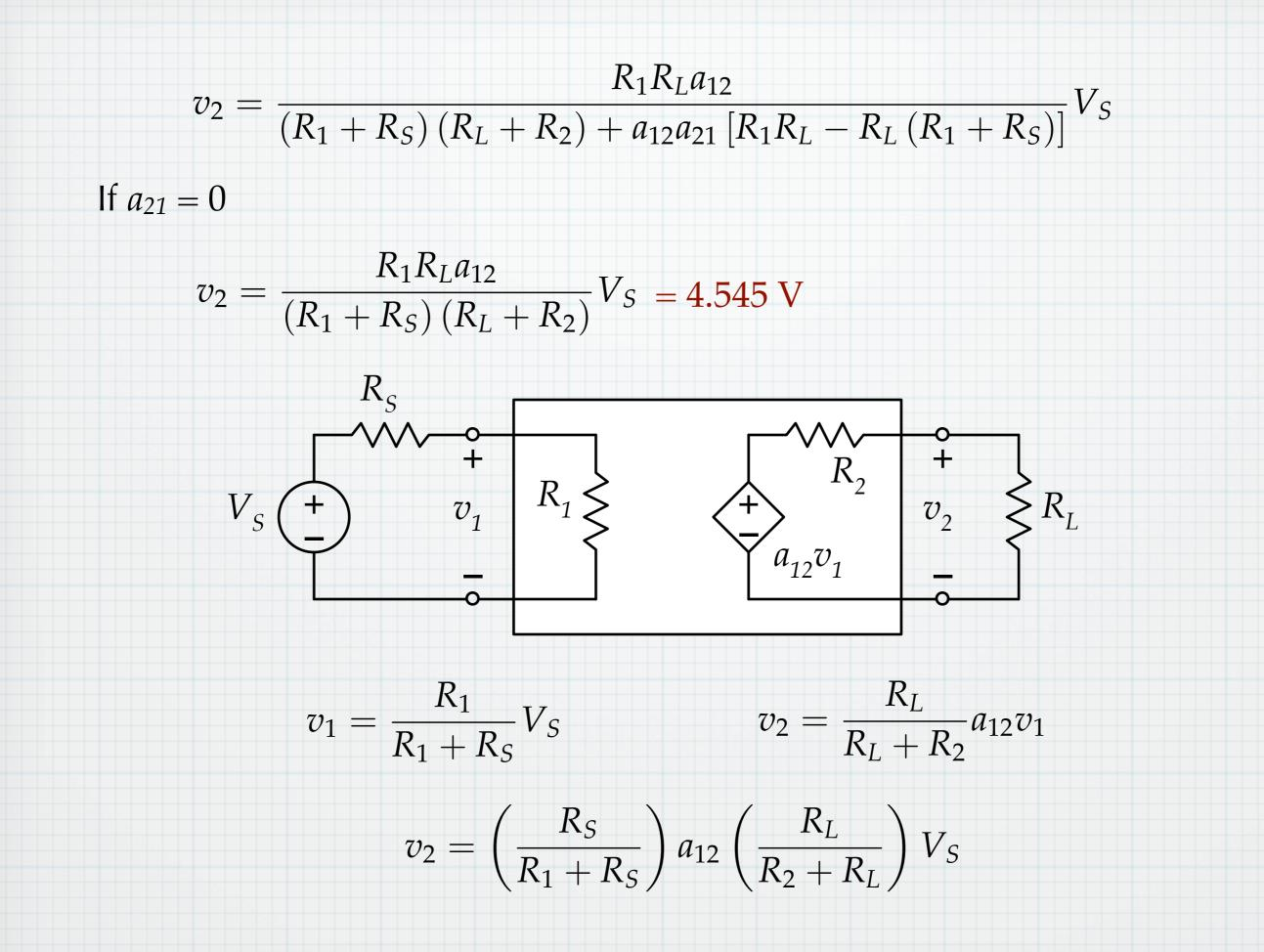
For amplifiers, the simpler model with  $a_{21} = 0$  is generally sufficient to provide a good description of the circuit's behavior.
