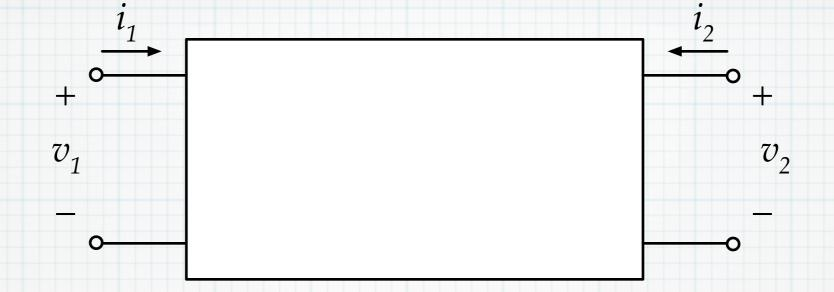
Express  $v_1$  and  $i_2$  terms of  $v_2$  and  $i_1$  (hybrid parameters)
