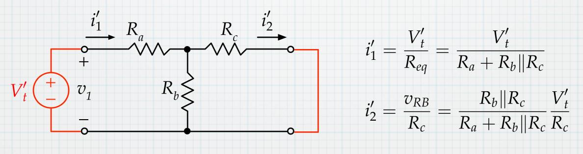
$$R_1 = \frac{V'_t}{i'_1} = R_a + R_b ||R_c = 1095\Omega \qquad \frac{R_2}{a_{12}} = \frac{V'_t}{i'_2} = R_c \frac{R_a + R_b ||R_c}{R_b ||R_c} = 1150\Omega$$
