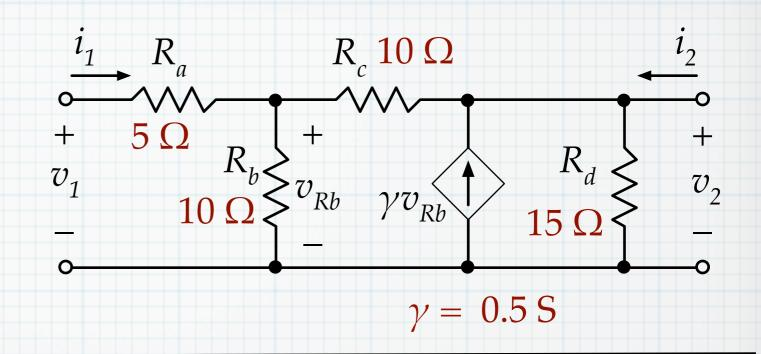
1. Short circuit  $v_{2}$  ( $R_d$  is shorted out.) Apply a test voltage at  $v_1$ . Calculate the terminal currents.
