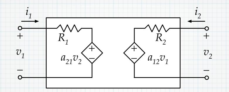
Need to use dependent sources. Now port 1 is connected to port 2 (the voltage at port 2 affects port 1) and vice-versa. This is the two-port version of the Thevenin equivalent idea. We can use this to model circuits that have an input and output.
