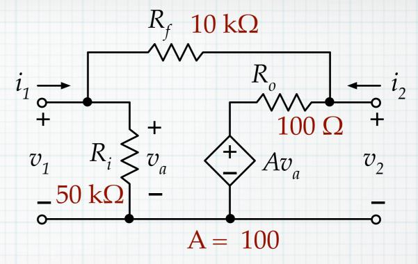
1. Apply a test voltage at  $v_1$ . Short circuit  $v_2$ . Calculate the terminal currents.
