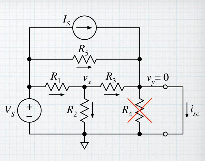
$$i_{sc} = \frac{3.385 \text{ V}}{1 \text{ k}\Omega} + 1 \text{ mA} + 6 \text{ mA}$$
