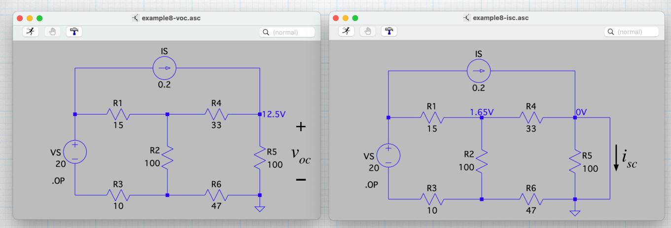
$V_{Th} = v_{oc} = 12.5 \text{ V}.$   $I_N = i_{sc} = 0.2 \text{ A} + (1.65 \text{ V})/(33 \Omega) = 0.25 \text{ A}.$
