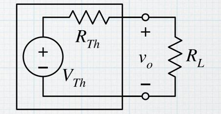
If we view the power as a function of  $R_L$ , we can find the maximum by using the usual calculus trick of taking the derivative and setting it equal to zero.
