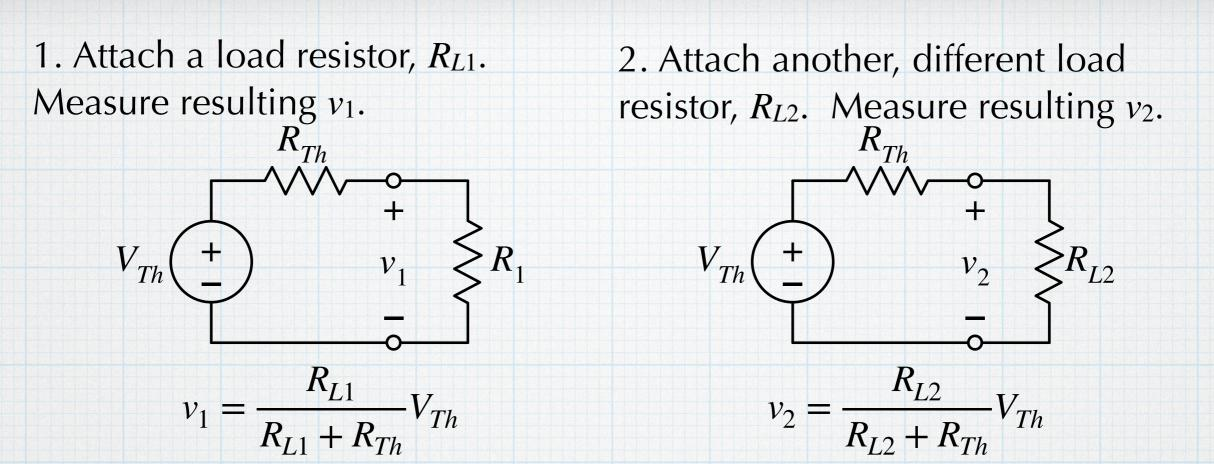
Knowing  $v_1$  and  $v_2$ , it is a simple matter to use the two equations to solve for the two unknowns,  $V_{Th}$  and  $R_{Th}$ .
