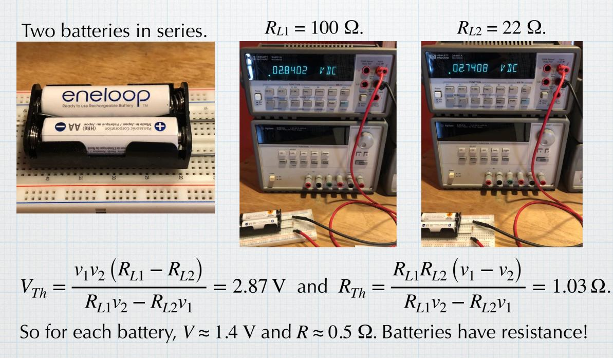
G. Tuttle <sup>1</sup> I frequently use this battery setup to power electronics circuits.
