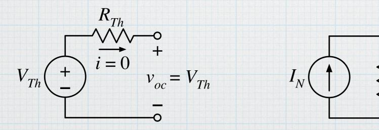
We still need a second measurement. What if we choose  $R_{L2}$  to be a short-circuit ( $R_{L2} = 0$ )? In the Norton circuit, we see that the short circuit at the load effectively shorts out  $R_N$  (no voltage across means no current through), and all of the source current must flow through the short,  $i_{sc} = I_N$ !
