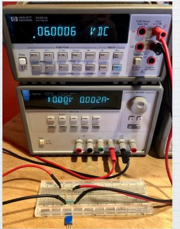
Insert pot. Adjust to  $v_{oc}/2$ .
