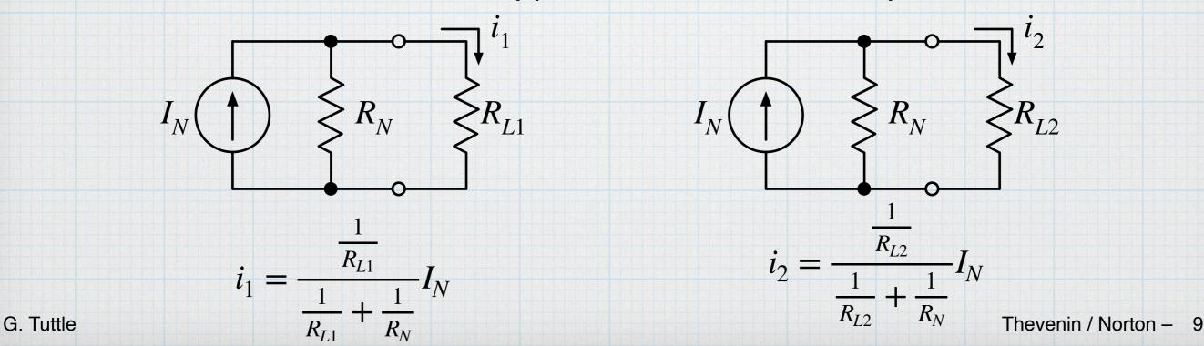
Now that we see the basic approach, we can apply it to other circuits. Attach a known load resistance and determine the corresponding port voltage. Then attach a second load and find the port voltage for that. Use the results to find the Thevenin (or Norton) equivalent for the circuit.
