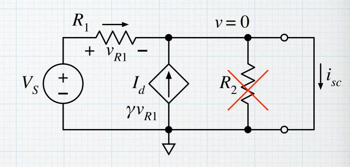
Note that if we had incorrectly tried to use the short-cut method for finding  $R_{Th}$ , we would have shorted the voltage source and then probably removed the dependent current source, leaving the two resistors in parallel. The result would have been "close-ish" to the actual value, but definitely not correct.
