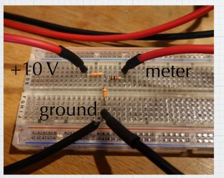
$$R_{Th} = \frac{6 \text{ V}}{2.61 \text{ mA}} = 2.30 \text{ k}\Omega$$
