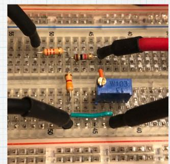
Pot removed. Measure *v*<sub>oc</sub>.
