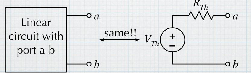
This view that every linear circuit has an effective voltage (which could be zero!) and an effective resistance completely changes the way that we look at circuits.
