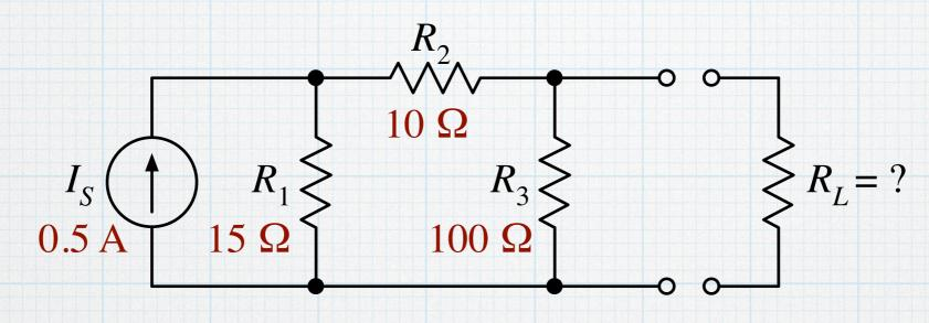
This is a Thevenin/Norton equivalent problem in disguise. Obviously, we need to find an equivalent circuit. We can start by finding the resistance. Since there is only a single  $R_1$ independent source, we can use the short-cut method. After deactivating  $I_S$ :
