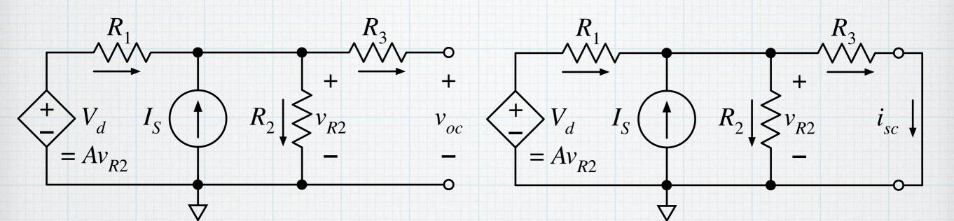
Find  $v_{oc}$ , which is equal to  $v_{R2}$ .
