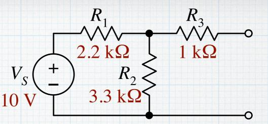
First, do the measurement in the lab. It's easy — just build the circuit on a breadboard with the 10-V supply for  $V_s$ . Use the multimeter at the port to first measure  $v_{oc}$  and then switch over to measure  $i_{sc}$ .
