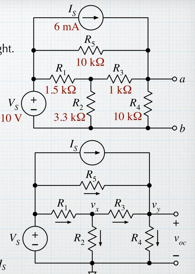
Inserting values and solving gives  $v_x = 11$  V and  $v_y = 15$  V. So  $V_{Th} = 15$  V.
