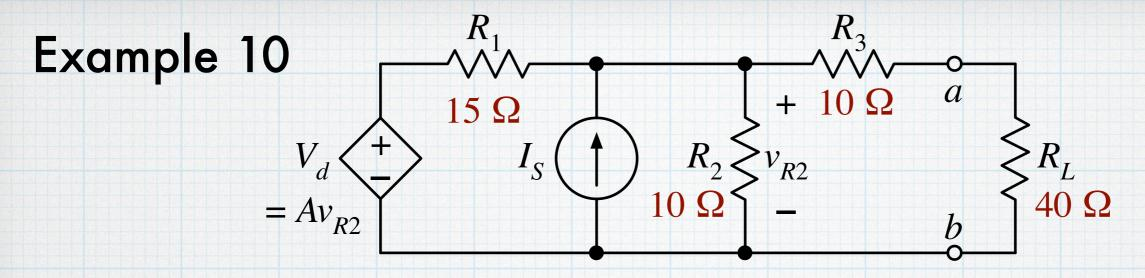
We are tasked with finishing the design of a small circuit that will be part of some electronic system. The basic topology is shown above. The circuit must have its equivalent resistance matched to the external 40- $\Omega$ load and be able to deliver 3.6 W to the load. Some of the internal resistors are already specified. Finish the design by choosing  $I_S$  for the current source and A for the dependent voltage source so that the circuit is delivering its maximum available power to the load.
