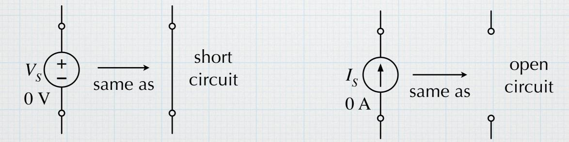
Replace voltage sources with shorts. Replace current sources with opens.
