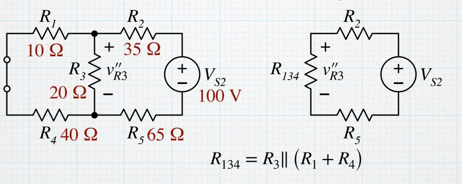
$$= (20 \Omega) \parallel (10 \Omega + 40 \Omega) = 14.29 \Omega$$
