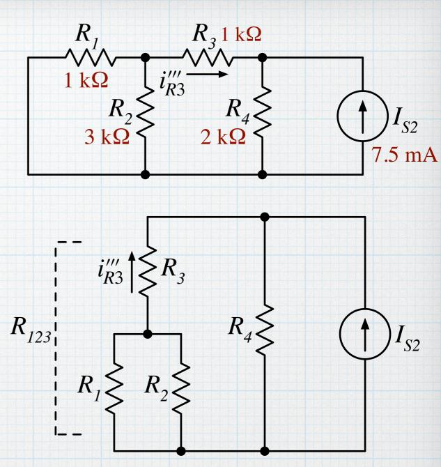
$R_{123} = R_1 ||R_2 + R_3 = 1 \,\mathrm{k}\Omega ||3 \,\mathrm{k}\Omega + 1 \,\mathrm{k}\Omega = 1.75 \,\mathrm{k}\Omega$
