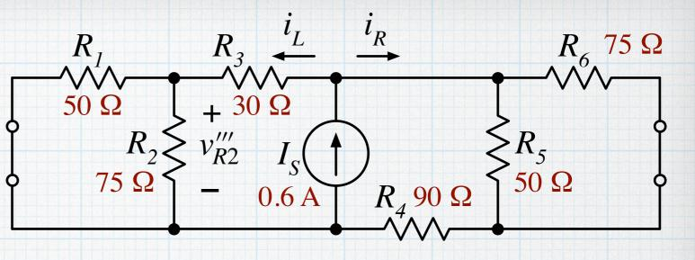
$$R_{L} = R_{3} + R_{1} || R_{2} \qquad R_{R} = R_{4} + R_{5} || R_{6}$$
