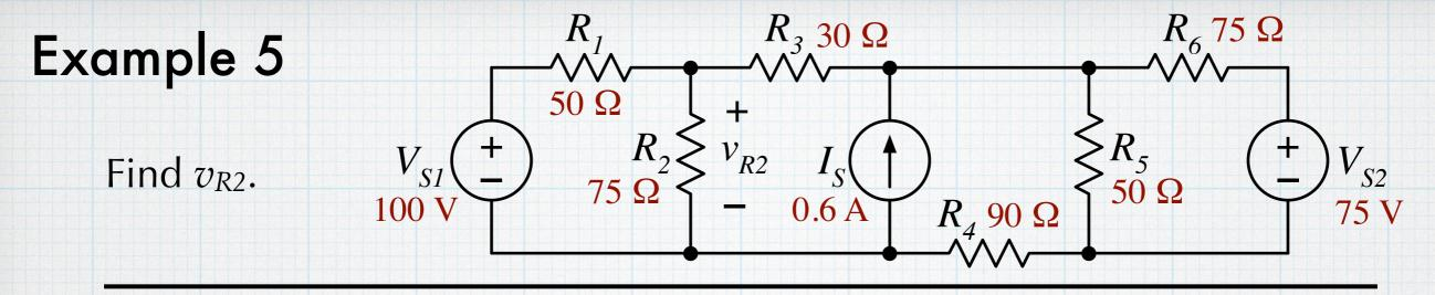
This looks nasty – there are 6 nodes with a super node or 4 meshes with a super mesh. Either NV or MC will be tough. We might be able to do a bunch of source transformations, but since there are only three sources, let's try superposition.  $R_1$ ,  $R_3$ ,  $R_6$
