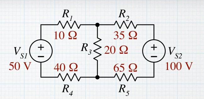
1. In using superposition, we cannot find "partial powers" — we need to find either total voltage or total current and then calculate power. For this problem, we will choose to find  $v_{R3}$ . Start by deactivating  $V_{S2}$ . We note that the series combination of  $R_2$  and  $R_5$  is in parallel with  $R_3$ .
