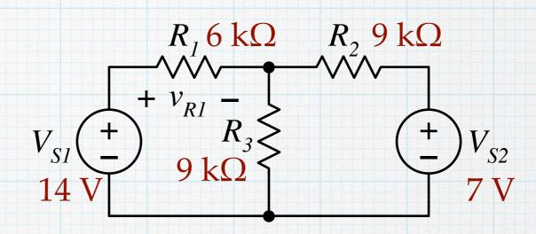
1. Deactivate  $V_{S2}$ . The result is a voltage divider between  $R_1$  and the parallel combination of  $R_2$  and  $R_3$ .
