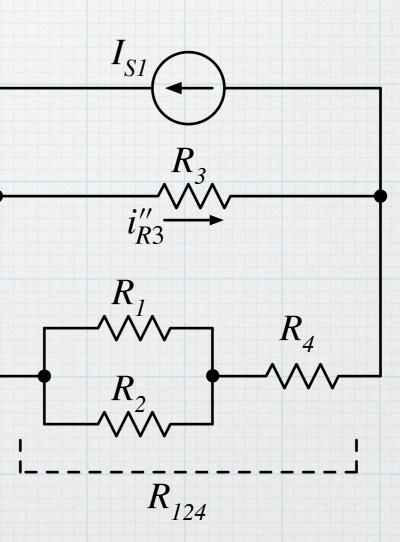
3. To obtain the final partial circuit, go back to the original circuit and deactivate *V<sub>s</sub>* and *I<sub>s1</sub>*, keeping *I<sub>s2</sub>*. As in the prior case, *R<sub>1</sub>* is in parallel with *R<sub>2</sub>*.
