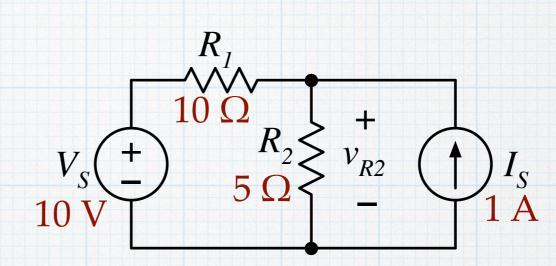
1. Deactivate (turn off) one of the sources — the order doesn't matter. Let's deactivate the current source first — set the value of *I*<sub>S</sub> to zero, which has the same effect as replacing *I*<sub>S</sub> with an open circuit. The result is a simple voltage divider, and we can easily calculate the partial result due to the voltage source.
