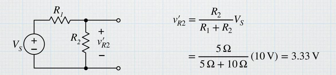
2. Go back to the original circuit and turn off the other source – set  $V_s$  to zero, which is the same as replacing it with a short circuit.
