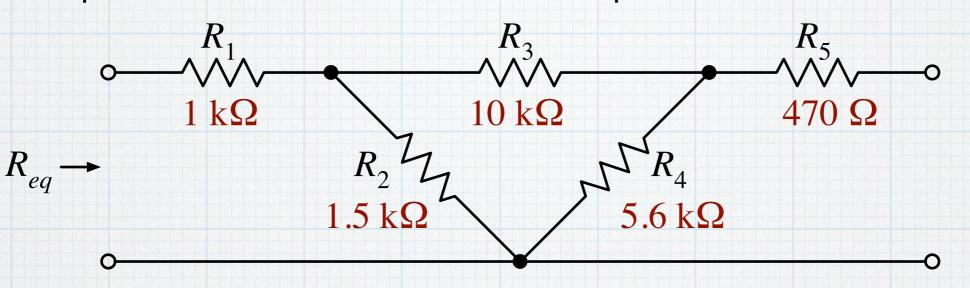
There are a couple of interesting things going on here. First, we see some "diagonal" resistors. Secondly, we see a "dangling" resistor,  $R_5$ , which is not connected to anything on one side.
