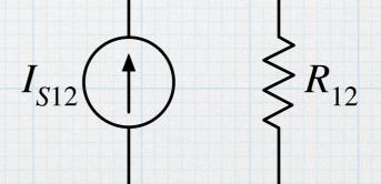
All the components have the same voltage across,  $v_{IS1} = v_{IS2} = v_{R2} = v_{R2} = v_{S}$ , We know that we can combine the parallel resistors, and it appears that we can combine the current sources as well.
