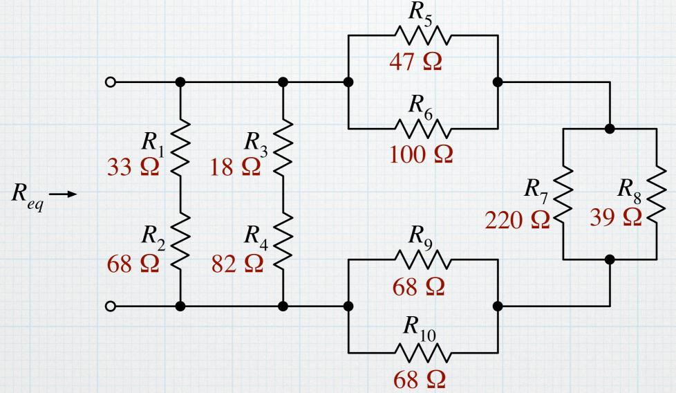
At first glance, this looks very difficult, but it's not so bad. We can pick it apart piece by piece. Start by noting that  $R_7$  is in parallel with  $R_8$ .
