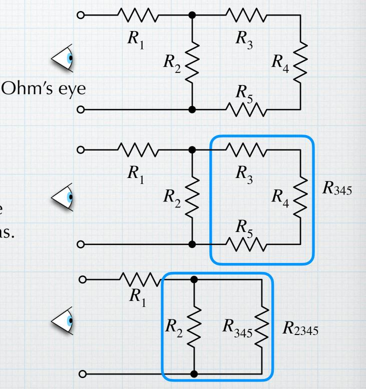
4. Continue the simplification process, one series or parallel combination at a time, until the network is reduced to a single resistor. (Or until the remaining network is trivial.)
