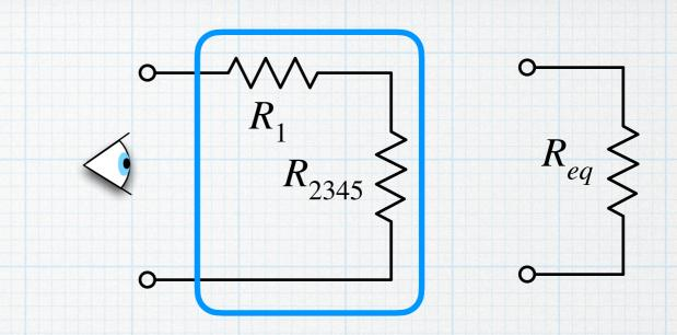
It is not necessary to insert numbers at each step — we could express the results using symbols and then insert numbers at the end, if needed. For the example, the equivalent resistance expressed in symbols:
