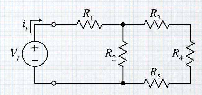
$R_{eq} = 10 \text{ V} / 5.02 \text{ mA} = 1.99 \text{ k}\Omega.$
