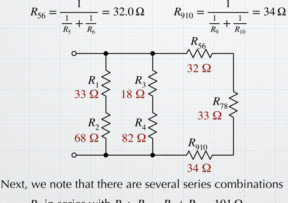
$R_1$  in series with  $R_2$ :  $R_a = R_1 + R_2 = 101 \Omega$
