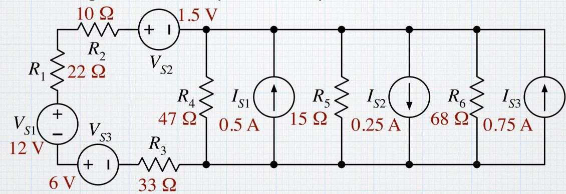
Three resistors in series on the left:  $R_L = R_1 + R_2 + R_3 = 65 \Omega$ Three sources in series on the left:  $V_L = V_{S3} + V_{S1} - V_{S2} = 14.5 \text{ V}$ Three resistors in parallel on the right:  $R_L$   $R_R = (R_4^{-1} + R_5^{-1} + R_6^{-1})^{-1} = 9.74 \Omega$ Three sources in parallel on the right:  $V_L$  $I_R = I_{S1} - I_{S2} + I_{S3} = 1 \text{ A}.$
