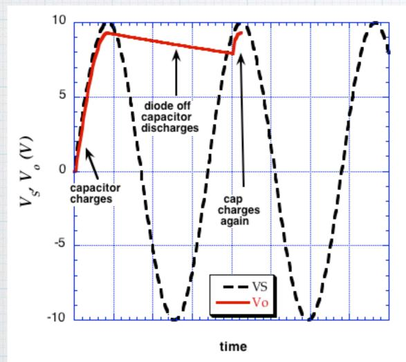
Diode stay off until  $V_S$  comes back around and becomes bigger than  $v_C$ . Then diode comes on again and re-charges the capacitor.
