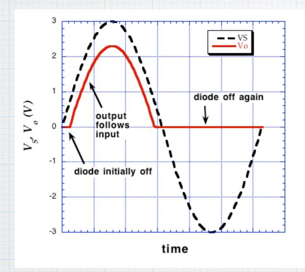
The diode turns off when  $V_S$  < 0.7 V. It stays off during the negative half cycle of the sinusoid.
