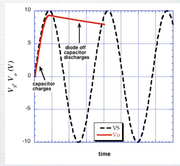
While  $V_S < v_{C_s}$  diode is off! Cap discharges through load.
