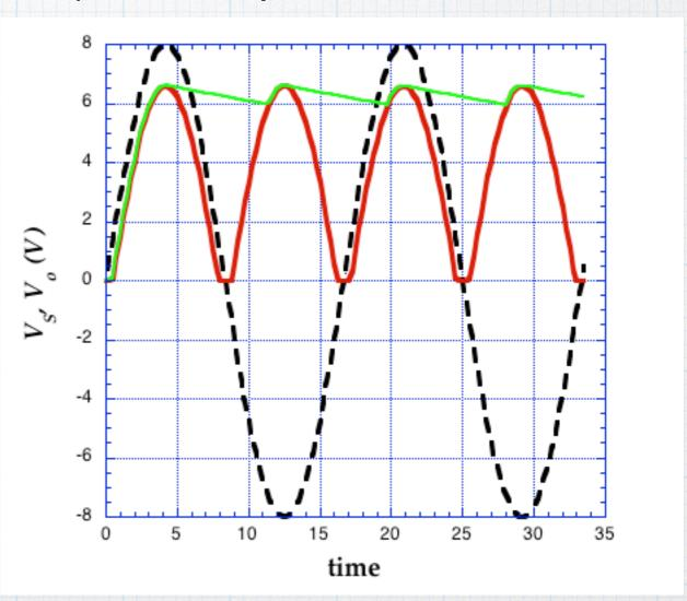
The ripple voltage is calculated in exactly the same way, except that the period is cut in half (frequency doubled).
