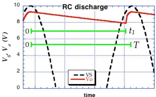
$t_1$  = time when diode conducts again.
