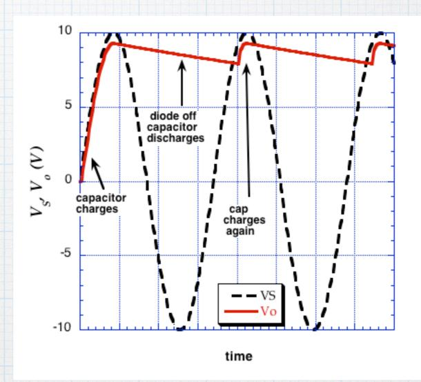
When  $V_S$  falls to less than  $v_C$ , the diode turn off again, and the cycle continues.
