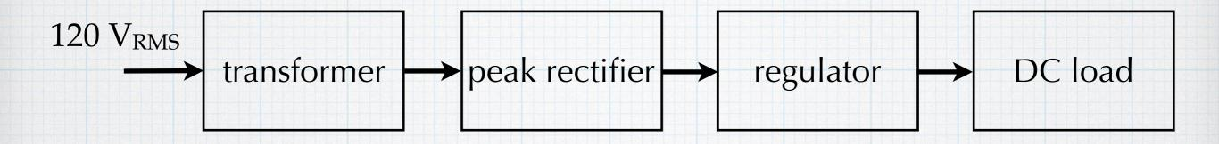
transformer: reduces AC amplitude to something safe and manageable.  $V_{peak}$  from the transformer will be a few volts bigger than the desired DC voltage.
