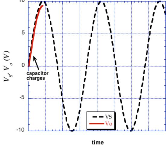
Initially, diode is on & cap charges to  $V_P$  - 0.7 V.
