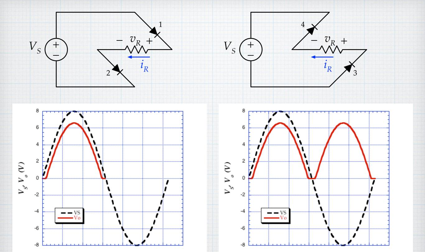
Note that there are no two diode drops in the conduction path(s). Also, the frequency is effectively doubled.
