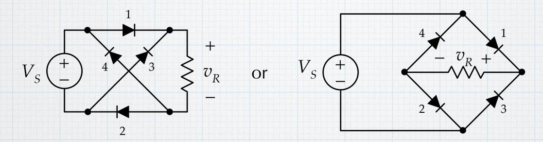
The diodes are in a bridge configuration.
