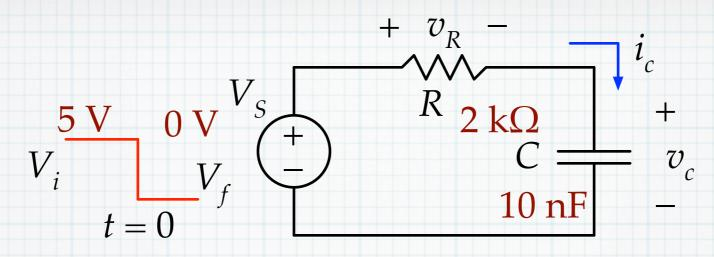
In the RC circuit above,  $V_s$  abruptly changes value from  $V_i = 5$  V to  $V_f = 0$  (essentially shorted out) at t = 0. Assume that the source was at  $V_i$  for a "very long time" before t = 0. Find the expression for the capacitor voltage as a function of time. Find the time at which  $v_c = 1$  V.
