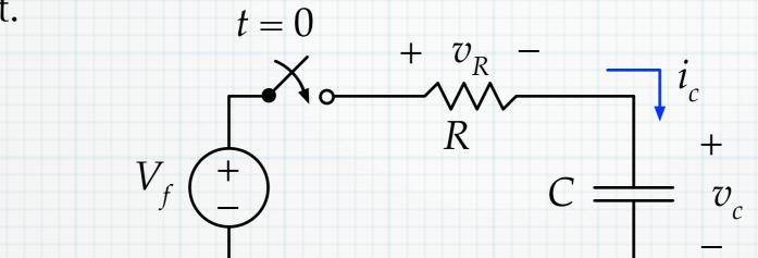
1. For t < 0, if the capacitor has some charge, it will have an initial voltage,  $v_c(t < 0) = V_i$ . Also,  $i_c = 0$ .
