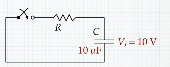
The capacitor above is charged to  $V_i = 10$  V. It is discharged by connecting a resistor in parallel (using a switch). Find the value of the resistor so that the capacitor is 90% discharged in 5 ms.
