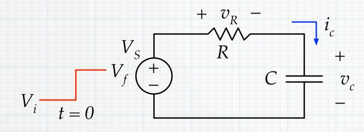
In the circuit,  $V_s$  abruptly changes value from  $V_i$  to  $V_f$  at t = 0. Assume that the source was at  $V_i$  for a "very long time" before t = 0.
