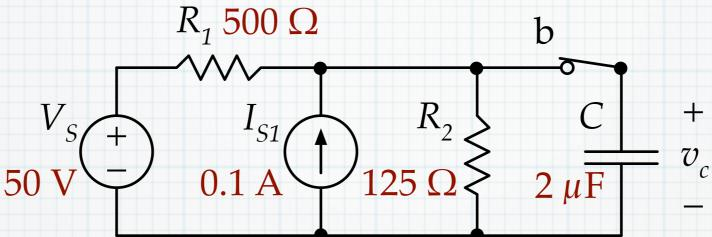
Find Thevenin as seen by capacitor. Use your favorite method. Note that  $V_{Th} = V_f$ .  $R_{Th} 100 \Omega$  $RC = 200 \ \mu s$  $2 \mu F$  $v_{c}(t) = V_{f} - \left[V_{f} - V_{i}\right] \exp\left(-\frac{t}{RC}\right)$  $= 20V - [15V] \exp\left(-\frac{t}{200\mu s}\right)$
