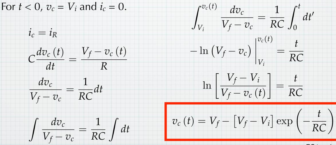
$$v_{c}(t) = V_{f} - \left[V_{f} - V_{i}\right] \exp\left(-\frac{t}{RC}\right)$$
