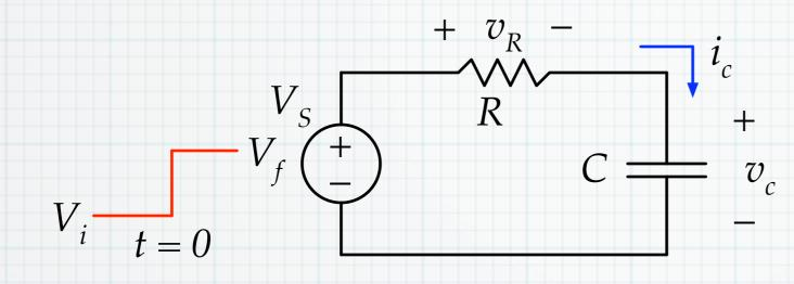
In the circuit,  $V_s$  abruptly changes value from  $V_i$  to  $V_f$  at t = 0. Assume that the source was at  $V_i$  for a "very long time" before t = 0.
