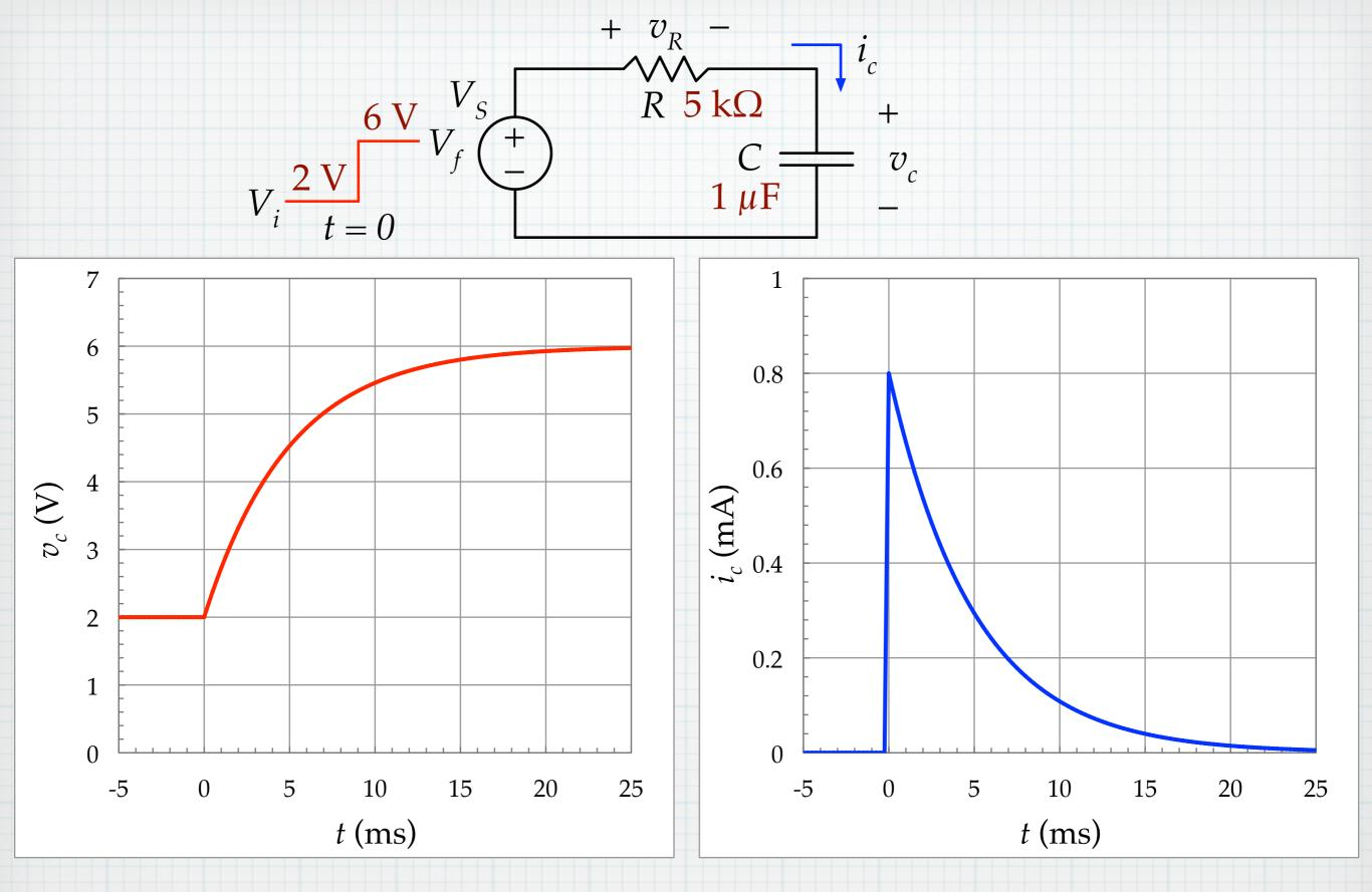
Plots of capacitor voltage and current for a simple *RC* circuit with  $V_f = 6 \text{ V}$ ,  $V_i = 2 \text{ V}$ ,  $R = 5 \text{ k}\Omega$ ,  $C = 1 \mu \text{F}$  (RC = 5 ms).
