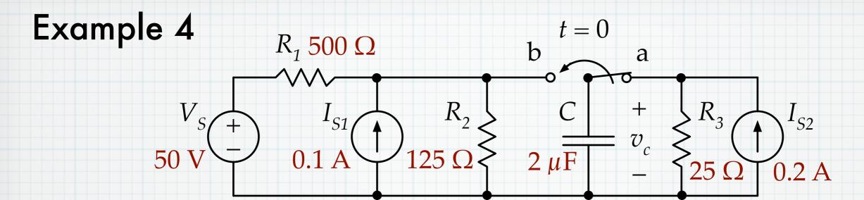
In the circuit above, the switch has been in position a "for a very long time". At t = 0, it abruptly switches to position b. Find the expression for the capacitor voltage as a function of time.
