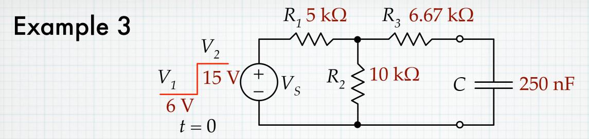
In the *RC* circuit above,  $V_s$  abruptly changes value from  $V_1$  to  $V_2$  at t = 0. Find the expression for the capacitor voltage as a function of time.
