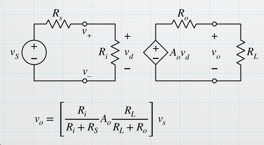
To minimize the effects of the input and output voltage dividers, we might try to make the input resistance be as big as possible — in the limit it would be open circuit — and the output resistance be as small as possible — in the limit it would be a short circuit.
