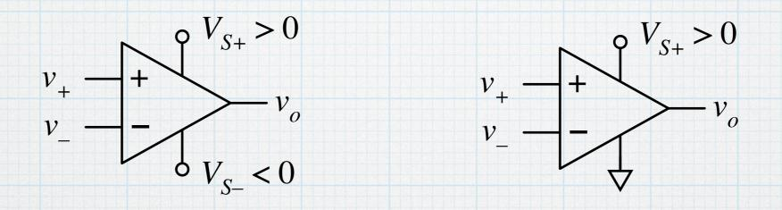
More typically, the power supply connections are not shown at all, as we did in all of the earlier examples. It is assumed that if the op amps are working, there must be power supplies available to make that happen.
