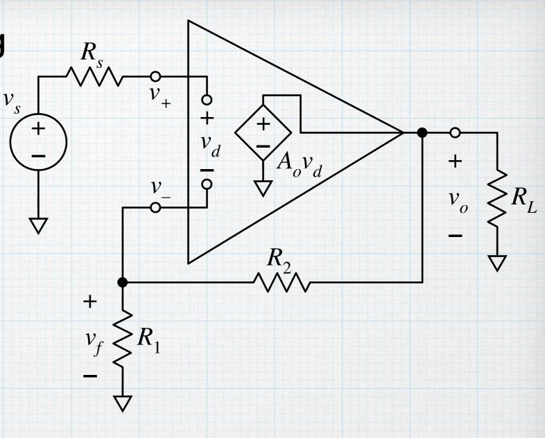
In drawing the circuit, we have made use of two bits of standard schematic nomenclature — the triangle symbol for the amplifier and the copious use of ground symbols. All the points with ground symbols form a single node. We could have connected all the ground points with wires, but the resulting schematic would have been almost un-intelligible. And this is a very simple electronic circuit. In more involved applications (EE 230), the schematics will have ground symbols all over the place.
