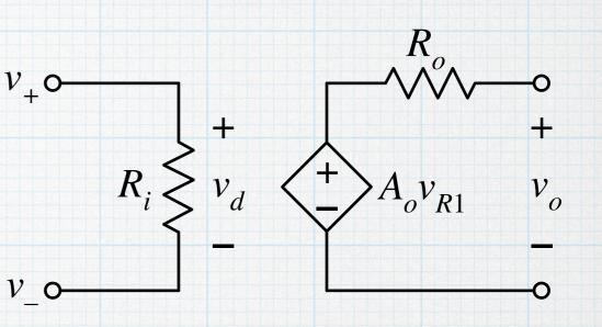
It is essential to specify all three parts of the model — when we attach an input source and an output load, the voltage developed across the load depends very much on  $R_i$  and  $R_o$ , as well as  $A_o$ .
