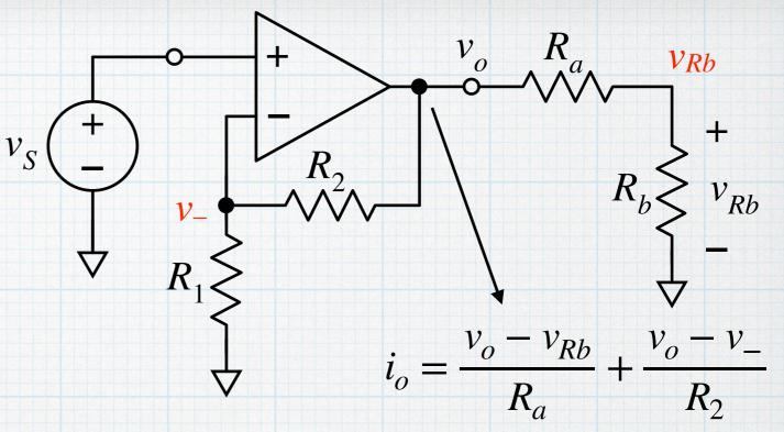
$\frac{v_o - v_-}{R_2} = \frac{v_-}{R_1} + i_- \text{ and } \frac{v_o - v_{Rb}}{R_a} = \frac{v_{Rb}}{R_b}$
