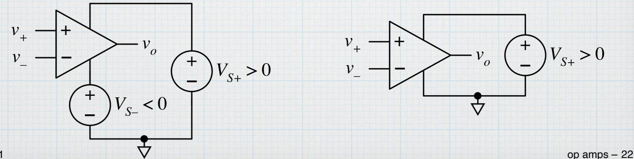
Including power supplies in the schematic become unwieldy, especially in circuits with multiple amps. Usually, the amps will share the same power supplies. If we want to show power supply connections explicitly, we can use the short-hand notation introduced earlier, where we simply label the voltages at the nodes.
