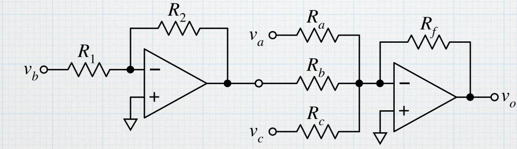
$$v_o = -\frac{R_f}{R_a} \cdot v_a + \left(\frac{R_f}{R_b}\right) \left(\frac{R_2}{R_1}\right) v_b - \frac{R_f}{R_c} \cdot v_c$$
