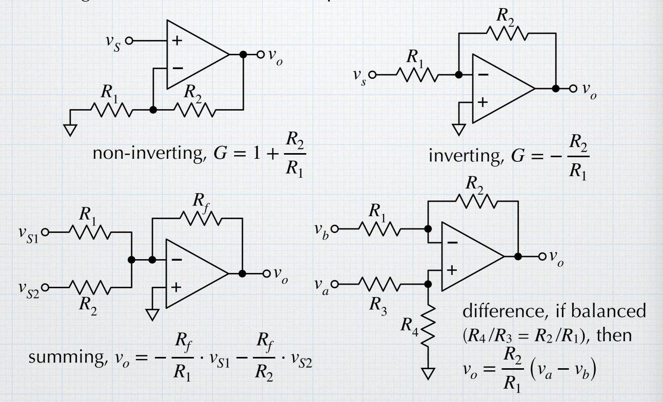
We can mix and match the basic configurations to achieve all sorts of circuit functions. The combining of op amp circuits works well because of the third feature of an ideal op amp: zero output resistance. With no output resistance, we can (in principle) connect anything to the output and not have to worry about mismatched input and output resistors affecting the voltage. If  $R_o = 0$ , the voltage divider ratio is always 1.
