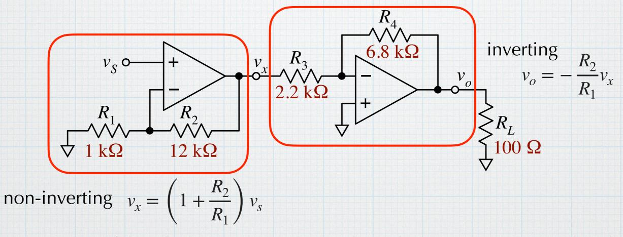
Because of the ideal output resistance, the voltage gains can considered piecemeal.  $\begin{pmatrix} R_4 \end{pmatrix} \begin{pmatrix} R_2 \end{pmatrix} = R_2 \end{pmatrix}$  The load resistor
