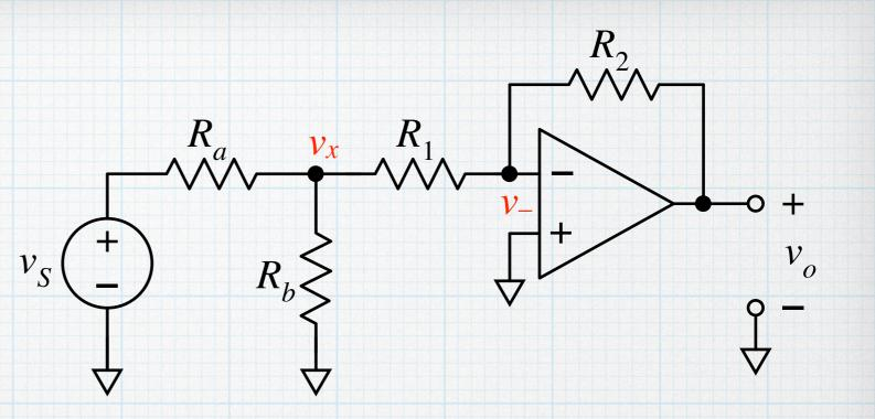
$$\frac{v_s - v_x}{R_a} = \frac{v_x}{R_b} + \frac{v_x - v_-}{R_1} \quad \text{and} \quad \frac{v_x - v_-}{R_1} = \frac{v_- - v_o}{R_2} + i_-$$
