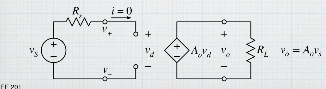
Op amps have a third distinguishing feature — a very large value for  $A_o$ . In the ideal case, the open-loop gain is assumed to be infinitely large! This would seem to cause some conceptual (and practical) difficulties, since then if  $v_d = v_s$  had any finite value, the output would go to infinity. The only way to keep the output from "blowing up" would be to have  $v_s = 0$ . This all seems a little odd.
