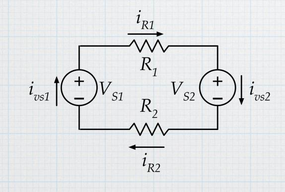
Applying KCL sequentially around the loop:
