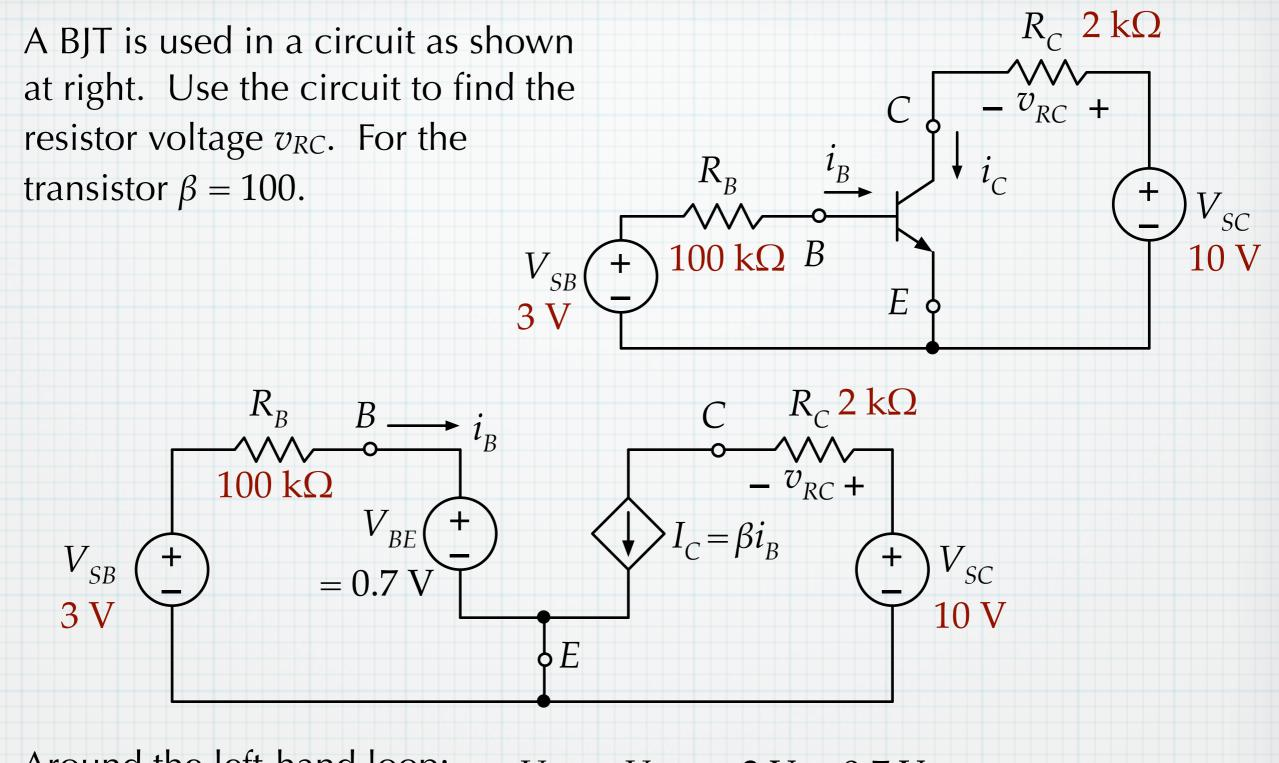
Around the left-hand loop:  $V_{SB} - i_B R_B - V_{BE} = 0.$   $V_{SB} - i_B R_B - V_{BE} = 0.$ On the right:  $I_C = \beta i_B = (100)(0.023 \text{ mA}) = 2.3 \text{ mA}.$
