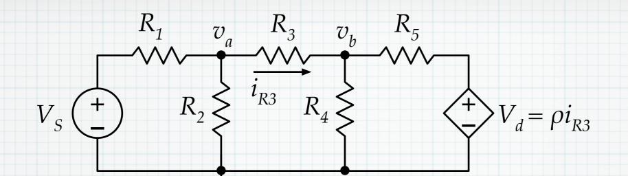
Write the node-voltage equations. (You should fill in the missing steps.)
