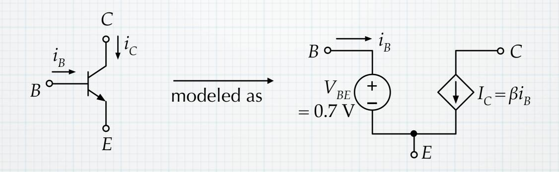
Even though it is fundamentally non-linear, in one particular mode of operation it behaves in a somewhat linear fashion and can be modeled using linear components, as shown at right. The primary feature of the BJT in this mode is current gain – a small current ( $i_B$ ) flowing in at one terminal leads to an "amplified" current flowing in another terminal.
