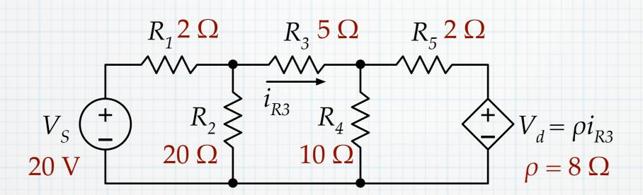
Use the node-voltage method. Define ground at the bottom and identify the unknown nodes. Initially, treat  $V_d$  as if it were known. We will write node equations for  $v_a$  and  $v_b$ , and then we add an *auxiliary* equation to handle  $V_d$ .
