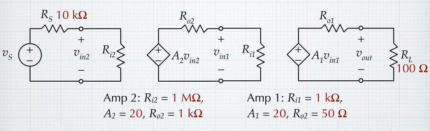
$$A_T = \frac{1M\Omega}{1M\Omega + 10k\Omega} (20) \frac{1k\Omega}{1k\Omega + 1k\Omega} (20) \frac{100\Omega}{100\Omega + 50\Omega} = 132$$
