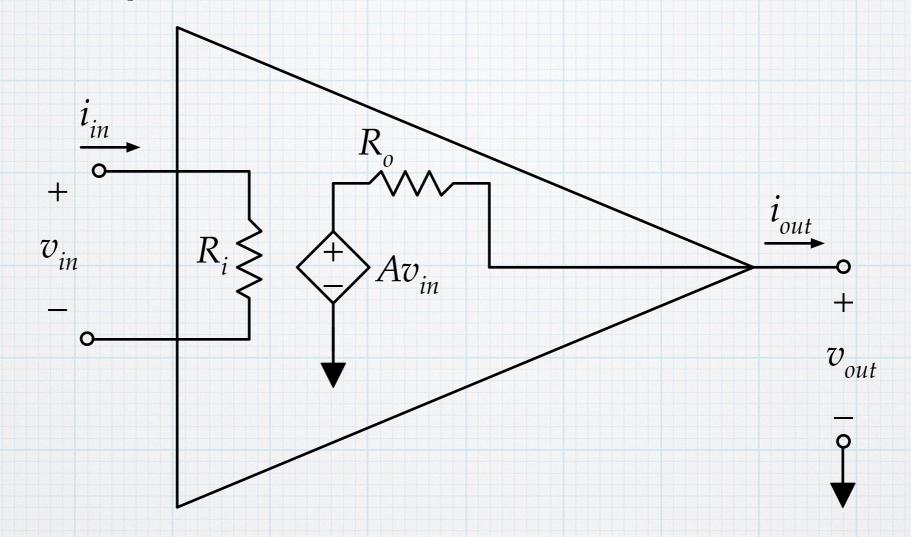
The usual circuit symbol for an amp is a triangle, with the input port at the base and the output port at the point. Many (most) amps use the circuit ground as one of the nodes defining the output port. So there is usually single output connection, and that output is referenced to ground. The ground in the circuit is defined by the DC power supplies that must connected to provide power for the amp to do its thing.
