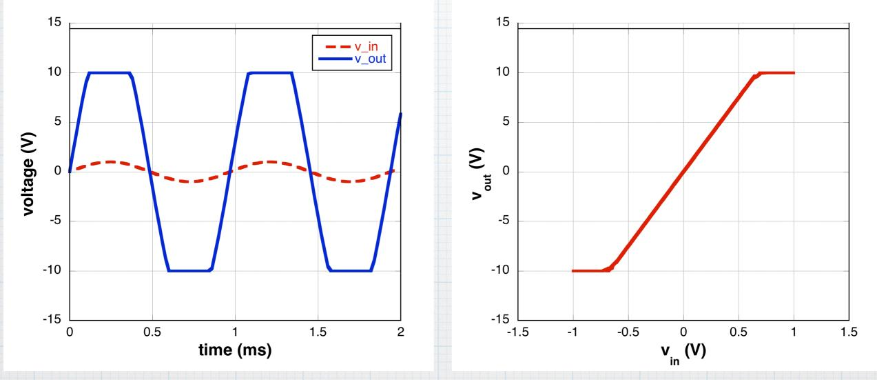
If input voltage and/or gain are too the bit, the output will "clip" at the limiting voltages. Since the output no longer has the same shape as the input, we say that it is "distorted". We will study this more later.
