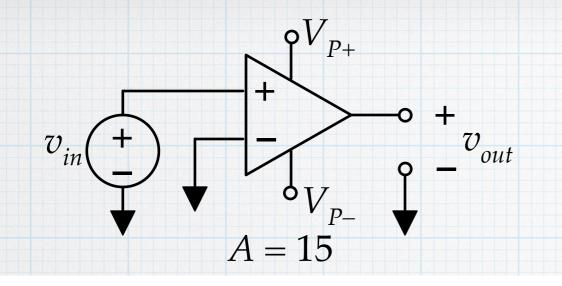
$v_{in} = (1 \text{ V}) \cdot \sin(2\pi f \cdot t)$   $v_{out} = A \cdot v_{in} = (15 \text{ V}) \cdot \sin(2\pi f \cdot t) \text{ (expected)}$ But if the power supplies limit at ± 10 V:
