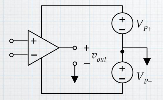
The power supply connections define the ground point in the circuit.
