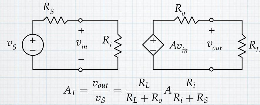
Ideally we would try to minimize the voltage lost across the voltage dividers, meaning that we make the divider ratio  $\rightarrow$  1. An ideal amplifier would provide the same gain independent of the source and load resistances.
