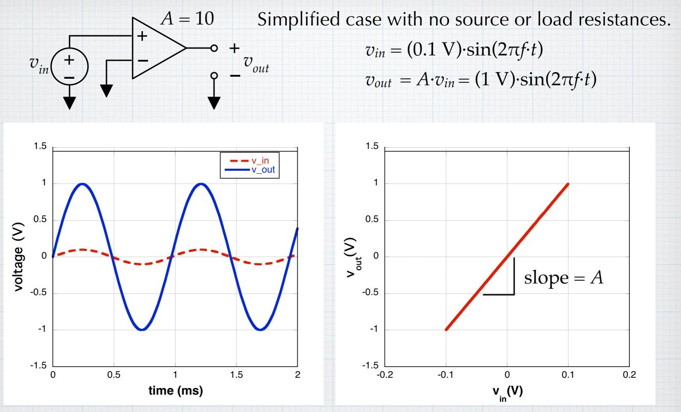
Two ways to represent the behavior of an amplifier. The plot on the left shows both  $v_{in}$  and  $v_{out}$  as functions of time. The plot on the right shows  $v_{out}$  as a function of  $v_{in}$ , which is known the *transfer characteristic*. Both plots can obtained easily with an oscilloscope.
