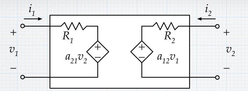
Take the basic two-port. Specialize it for an amplifier, which is usually designed to work in one direction only.
