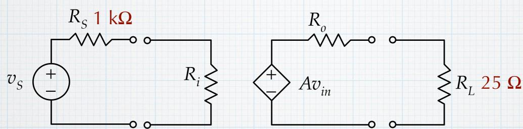
Amp 1:  $R_i = 500 \Omega$ , A = 60,  $R_o = 75 \Omega$
