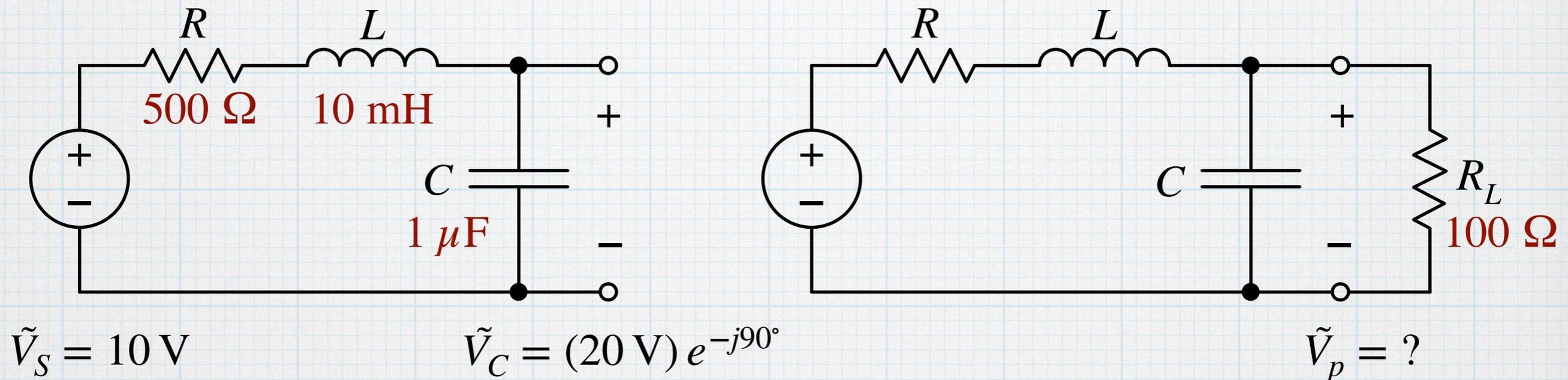
We immediately see the problem as we start the AC analysis. The extra resistor changes the impedance:
