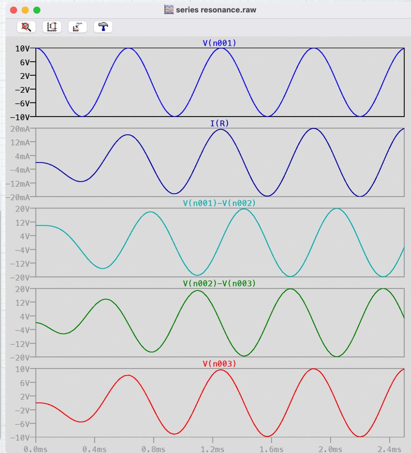
From top to bottom:  $v_S(t)$ ,  $i(t)$ ,  $v_C(t)$ ,  $v_L(t)$ , and  $v_R(t)$ .
