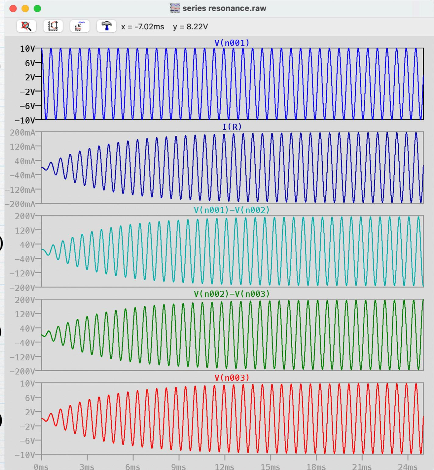
If the resistance is increased, say to  $R = 5 \text{ k}\Omega$ , so that the transient is no longer underdamped, we still see resonance,  $v_R = v_S$  and  $v_C = -v_L$ .
