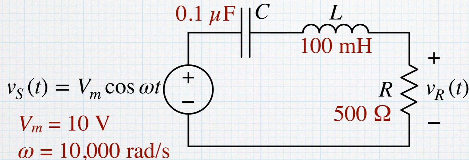
The complex voltage on the resistor is easily found using a voltage divider with the three impedances:  $Z_C$ ,  $Z_L$ , and  $Z_R$ .
