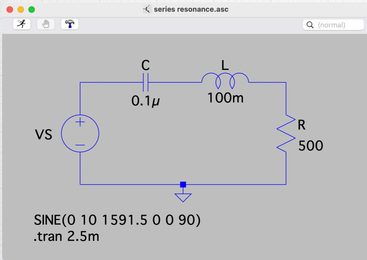
Note regarding SPICE: The frequency 1591.5 Hz corresponds to 10 krad/s. Also, we added a 90° phase shift to make a cosine rather than a sine in order to match with the hand analysis.
