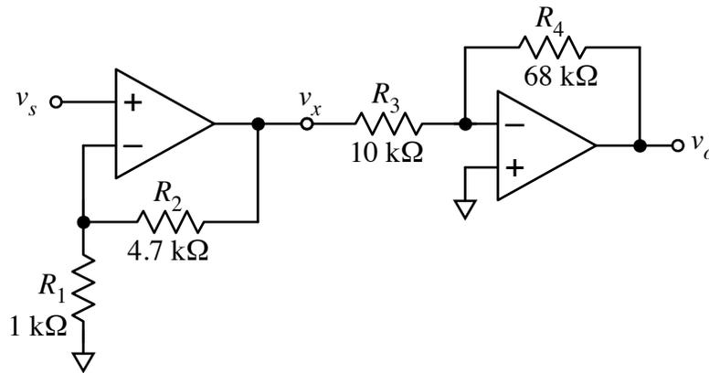
For  $v_s$ , use the function generator set to a sinusoid with frequency of 1000 Hz and amplitude of  $0.25\text{ V}_{\text{RMS}}$ .
