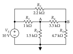
Figure 2. Node-voltage circuit B.
