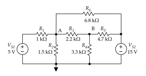
Figure 3. Node-voltage circuit C.
