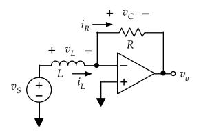
Apply a sinusoidal input:  $V_m = 1$  V (= 2 V peak-to-peak = 0.707 V<sub>RMS</sub>) and  $\omega = 10,000$  rad/s (f = 1560 Hz). Use the oscilloscope to observe the input voltage (i.e. inductor voltage) and output voltage (i.e. inductor current) simultaneously. Note the amplitude of the inductor current. Confirm that it matches expected value from the inductor i-v relation. Note the 90° phase shift between the voltage and current. Save a copy of the traces for your report.
