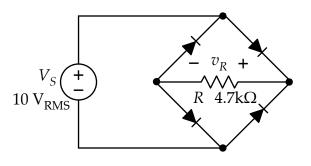
(a) Use SPICE to simulate the circuit and make a plot of the rectified resistor voltage as a function of time. Use a transient simulation with a sinusoidal source. Run the transient for at least 4 periods (of the source) in order to clearly see the ripple voltage.
