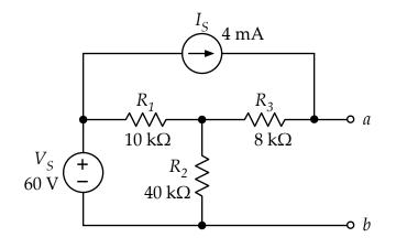
Find the Thevenin equivalent of the circuit with respect to terminals *a* and *b*, as shown below.
