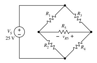
a. Calculate the voltage across  $R_5$ , if all five resistances are equal to 100  $\Omega$ .
