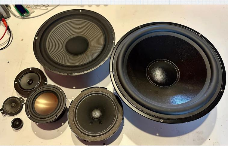
It is possible to use a single driver to cover the entire frequency range — a medium-sized mid-range could do a passible job. But it will not produce high-quality sound, since the low and high ends will be diminished. There will be less bass and treble. The sound will be recognizable, but it will not be "good".
