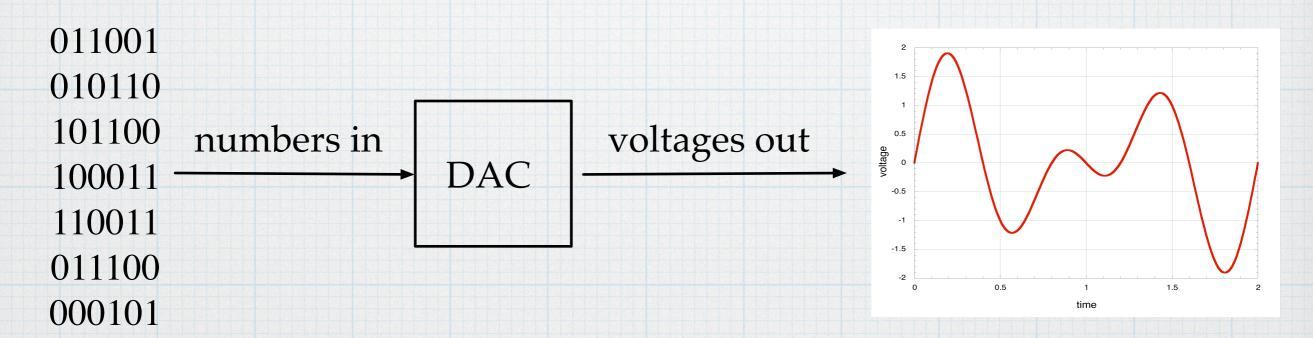
• Often the digital data is stored in a "lossy" format (mp3, aac, or similar) and must be converted back to a native format before using the DAC. (Digital signal processing, EE 424).
