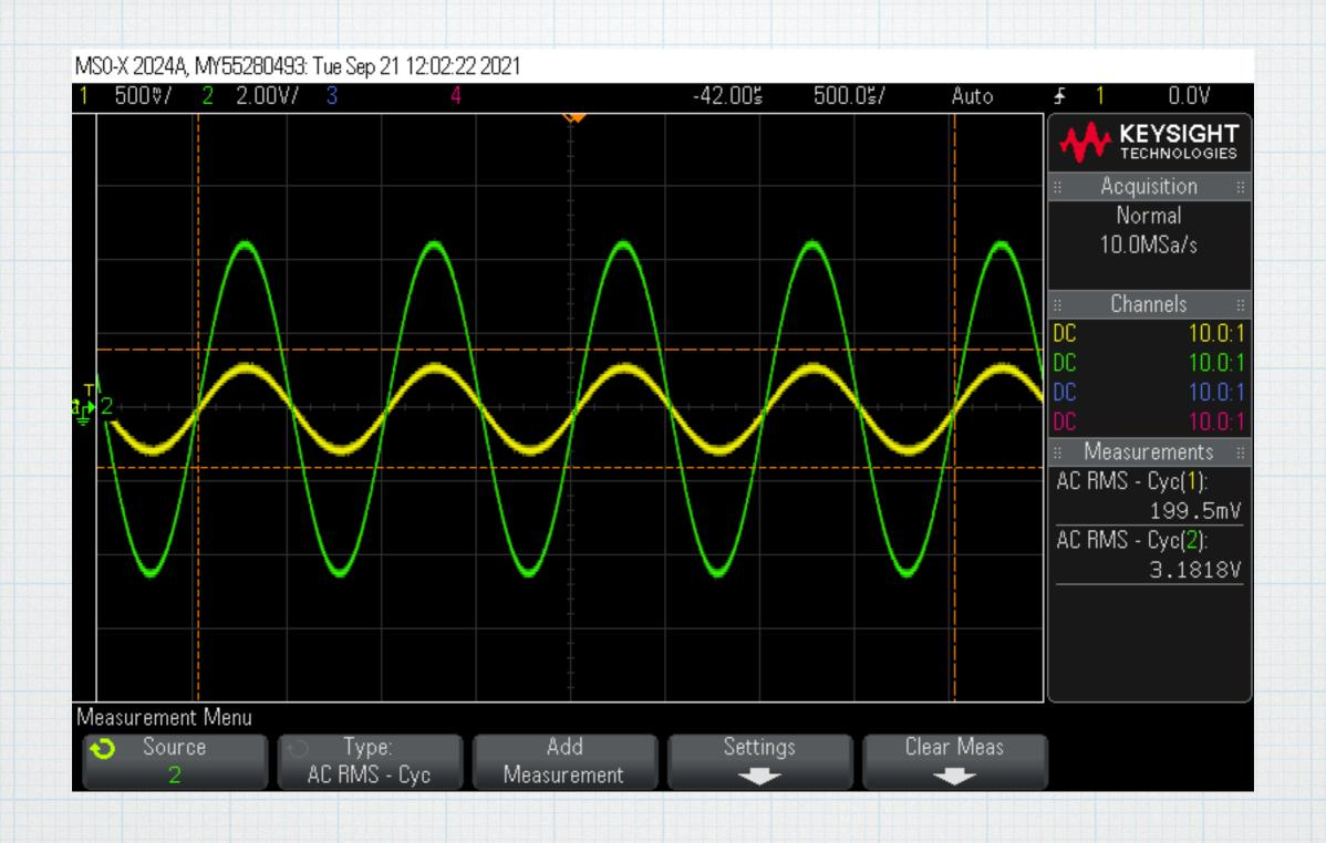
$$G = \frac{v_o}{v_i} = \frac{3.18 \text{ V}}{0.200 \text{ V}} = 15.9$$
