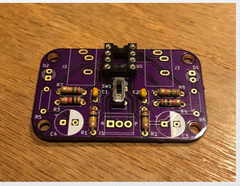
7. Battery connector Solder in the screw terminals for the battery connections. The center pin is connected to ground — be patient and turn up the temp if needed.
