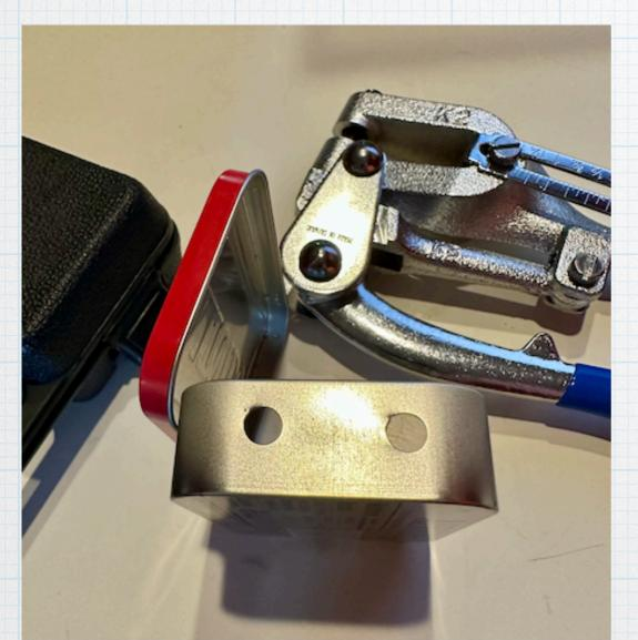
Since the holes are offset slightly from the center, it might be necessary to nip two small chunks out of the lid in order to have it close completely. G. Tuttle – 2023
