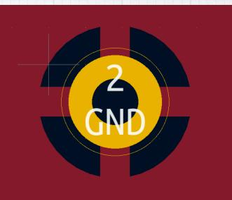
The thermals help, but it will still be more difficult to make solder connections to the ground plane. It will be necessary to get more heat into the connection to melt the solder. Things to do:
